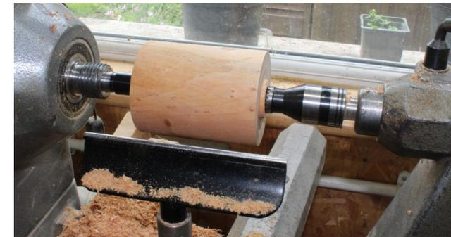
After turning to a cylinder, measurements taken from the scale drawing were used to shape the plinth to the required size.
