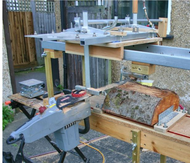
The first step was to cut the wood into manageable slabs using an electric chainsaw mill.
