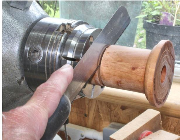
Using a pull saw to separate the plinth from the spigot
