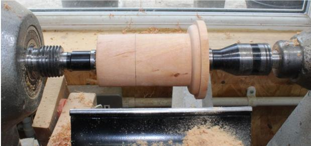
Here the base and the sides of the plinth have been shaped with bowl and spindle gouges.
