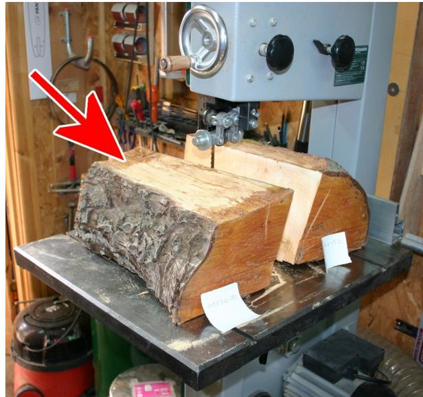
After slabbing with the chainsaw, it was further cut into turning blanks using a bandsaw. The arrowed block, after more trimming, became the turning blank for the plinth.
