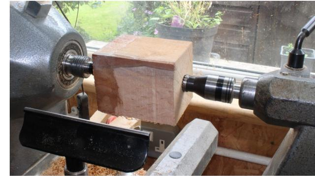
The rough cut turning blank mounted on the lathe (between centres) for making the plinth.
