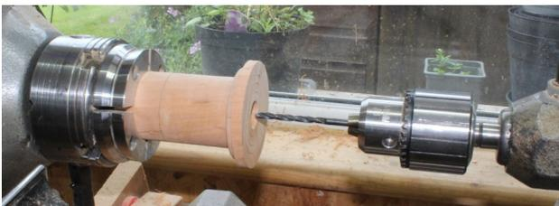
A 5mm diameter hole was then drilled right through to enable the trophy attachment bolt to pass through the top of the plinth into the recess.
