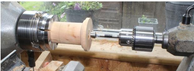
With the wood securely held in the lathe chuck, a recess of 20mm diameter was drilled to a depth of 30mm in the base of the plinth, using a Forstner drill bit.
